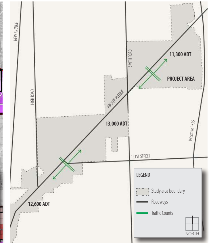
Figure 2: The Route 171 corridor has traffic counts that do not support the type of commercial development that the Comprehensive Plan envisions. Retailers prefer counts greater than 20,000 ADT, almost twice the current volume.
